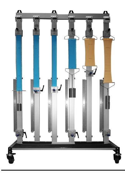
An accurate and flexible instrument for testing the stretch, growth and recovery properties of knitted and woven fabrics.
